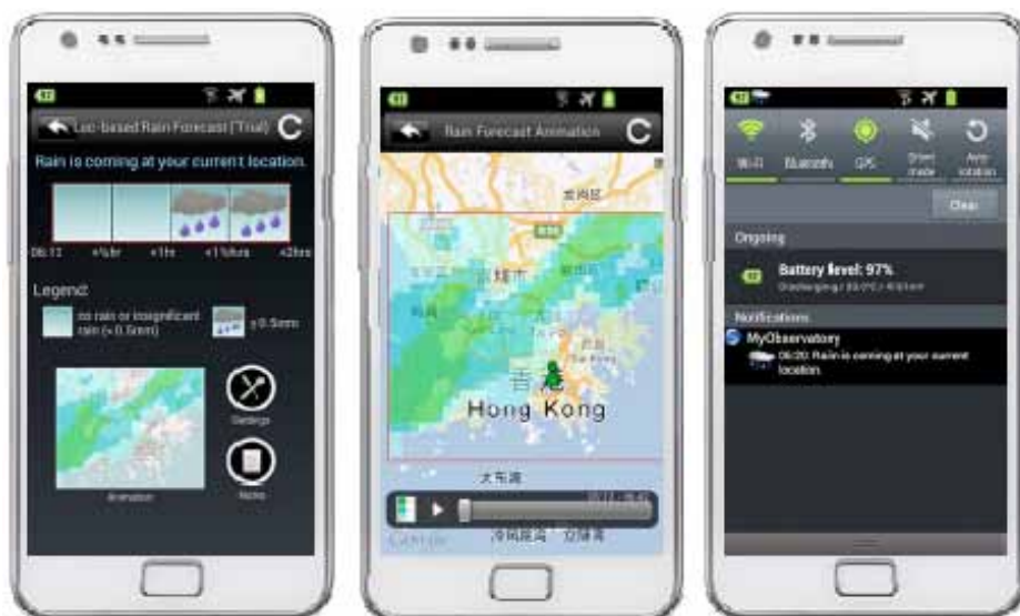
Figure 5 Sample screens for Location-based Rain Forecast service: (a) text and weather icon sequence (b) animated rainfall forecast map (c) notification message
